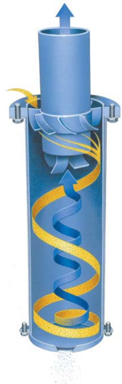
Operation of collecting tube assembly.
